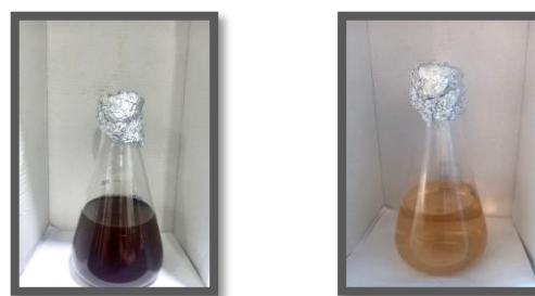
B- Extract after adding silver nitrate A-Extract before adding silver nitrate Figure1. Synthesis of silver nanoparticles by bacterial aqueous extract.
