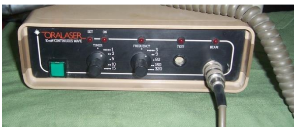
Figure (1) Gallium-Aluminum-Arsenide diode laser
