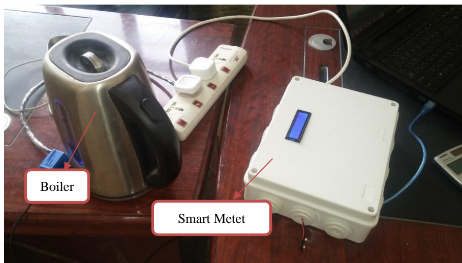
Figure 9. Testing of the Manufacturing Meter System via boiler connection
