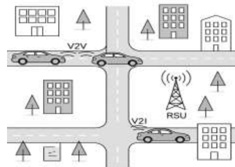
Fig. 1: Representative Vehicular Ad-Hoc Network showing V2V links, RSU-mediated V2I links
