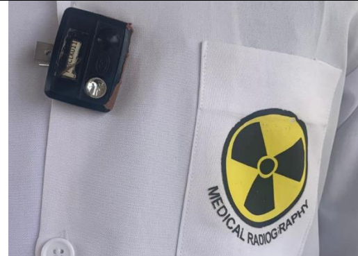
Fig. 3. Similar TLDs are used for the exam and for personal radiation monitoring
