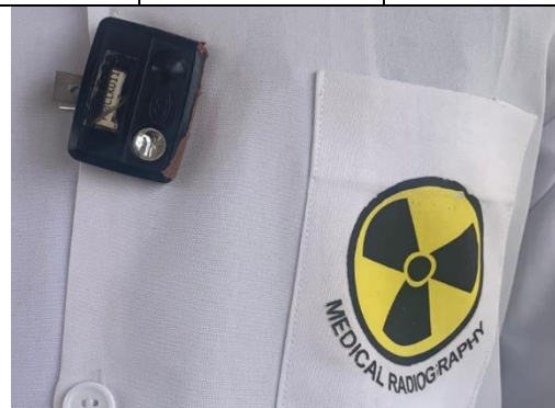
Fig. 3. Similar TLDs are used for the exam and for personal radiation monitoring
