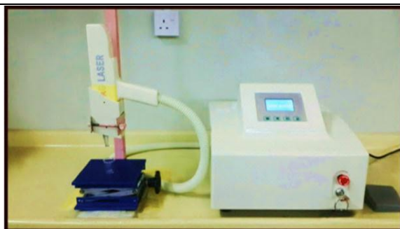
Figure 1: Experimental setup for nanoparticles synthesis by PLAL
