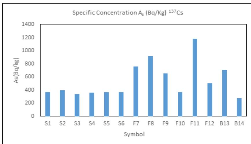
Figure (3): Comparison of the specific concentration of  $^{137}\text{Cs}$  in the study region samples
