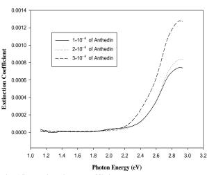
**Fig.(4):Extinction coefficient vs. wavelength** of concentrated epoxy with Al-Anthidendye
