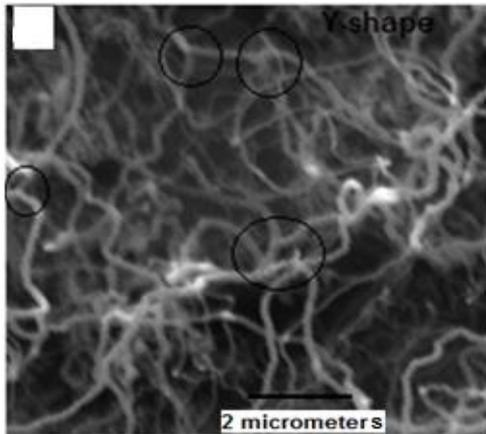
Fig.6. SEM for CNTs –CVD deposition on Si (100) coated with 170 nm Au film.
