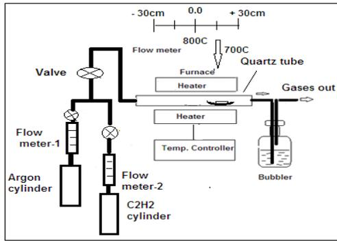
Fig.2 Schematic diagram of CVD system
