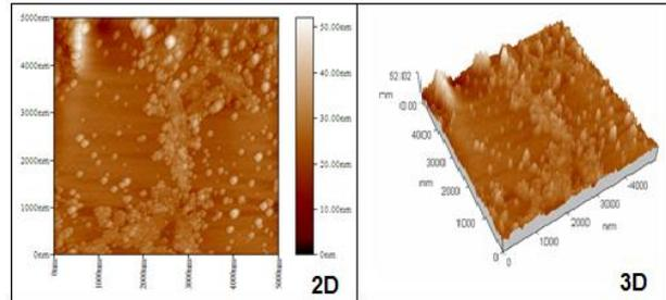
Fig. 3. AFM images in 2D and 3D for 140nm thick gold nanoparticles as deposited.
