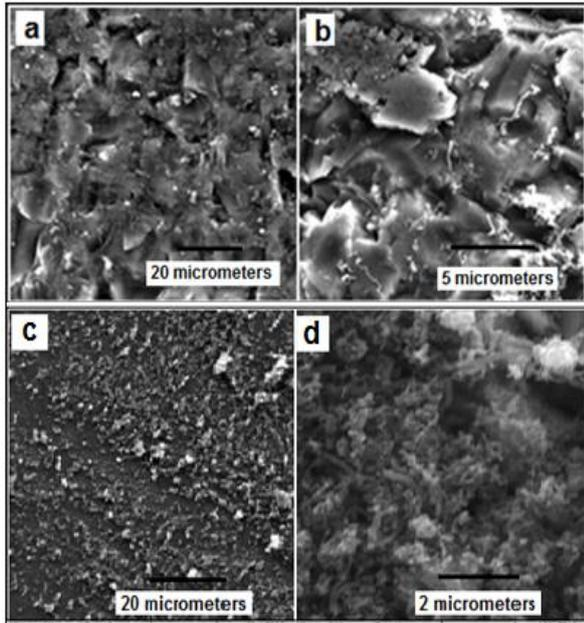
Fig.4. SEM images (top view) of as-synthesized carbon nanostructures as deposited on Si(100) coated with gold catalyst ( 10nm (a) ; 20nm (b) ; and 80nm (c and d). at different magnifications .
