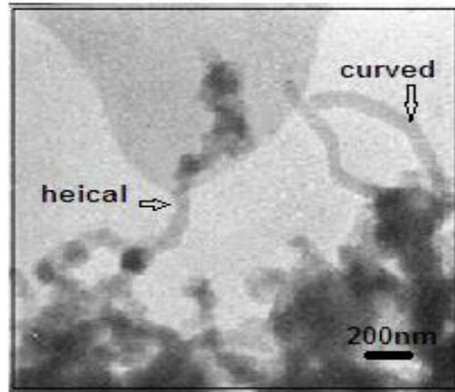
Fig.7 TEM image of CNFs grown at 800°C by CVD with 280nm gold catalyst on Si(100)
