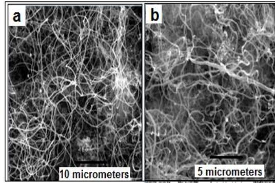
Fig.5 a,b. SEM images of CNFs with different area and magnification(140nm gold film).
