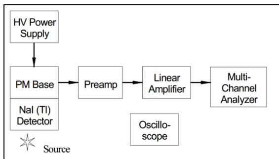
**Figure (1): Block diagram for a scintillation detector system [5]**
