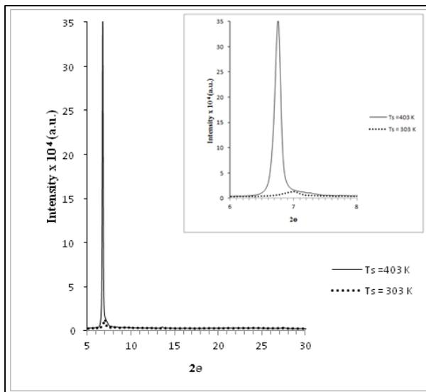
**Fig. 3. XRD pattern of CuPc thin films deposited at 303 °K and 403 °K**
