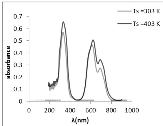
**Fig.1. Absorption spectra of CuPc thin films which prepared at both substrate temperatures (303 oK and 403 oK)**
