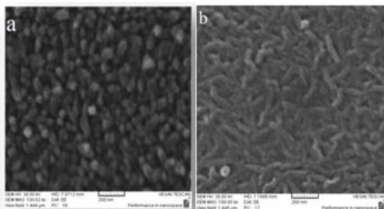
**Fig. 2. SEM image of Nano-structure CuPc grown on glass substrate at both substrate temperatures (a) 303 oK (b) 403 oK**
