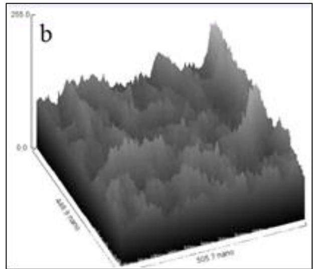
**Fig.4. AFM images of CuPc thin films deposited at Ts=303 °K in a) and Ts=403 °K in b)**
