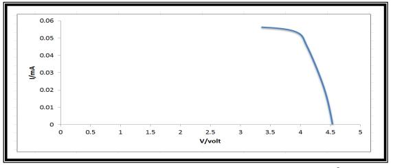
Figure (11) Current-Voltage curve solar cell using AuramineOdye( $2 \times 10^{-5}$ )mol/L of(0.32)mm thickness.
