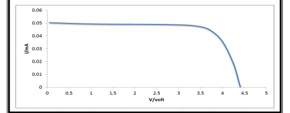
Figure (9) current – voltage curve solar cell using Auramine O dye $(1 \times 10^{-5})$  mol/Lof (0.21)mm thickness.
