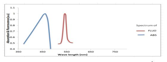
Figure(5)Absorption and Fluorescencespectra for AuramineOof( $5 \times 10^{-5}$ ) mol/L
