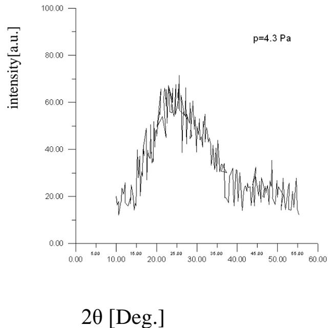
Fig. (5) XRD spectra of TiO<sub>2</sub> deposited at sputtering pressure(4.3 pa) andO<sub>2</sub>/Ar percentage (5%).
