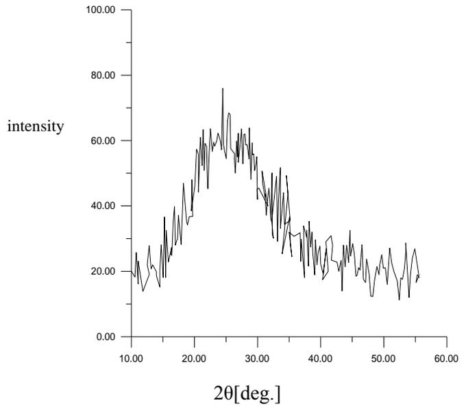
Fig. (4) XRD spectra of TiO<sub>2</sub> deposited at sputtering pressure(3.8 pa) andO<sub>2</sub>/Ar percentage (5%).
