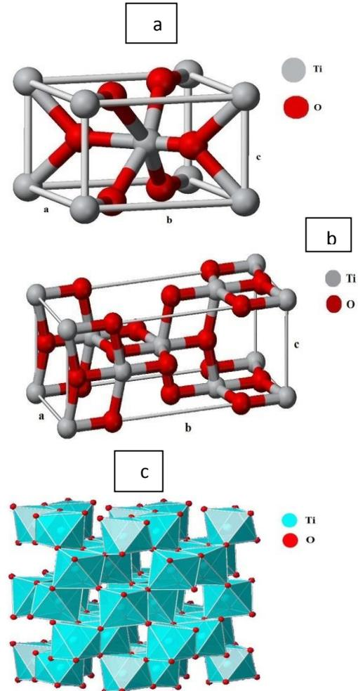
Fig. (1) a. Rutile structure for crystalline  $\text{TiO}_2$ . b. Anatase metastable phase for crystalline  $\text{TiO}_2$ . c. Brookite structure for crystalline  $\text{TiO}_2$  [3].
