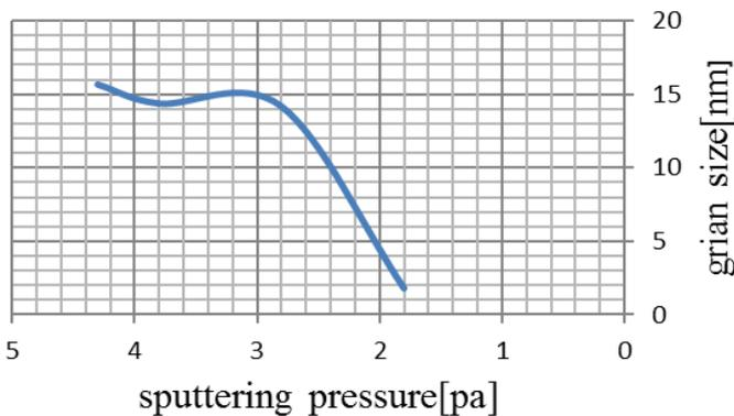
Figure (7) grain size as a function of sputtering pressure at O<sub>2</sub>/Ar percentage (5%).
