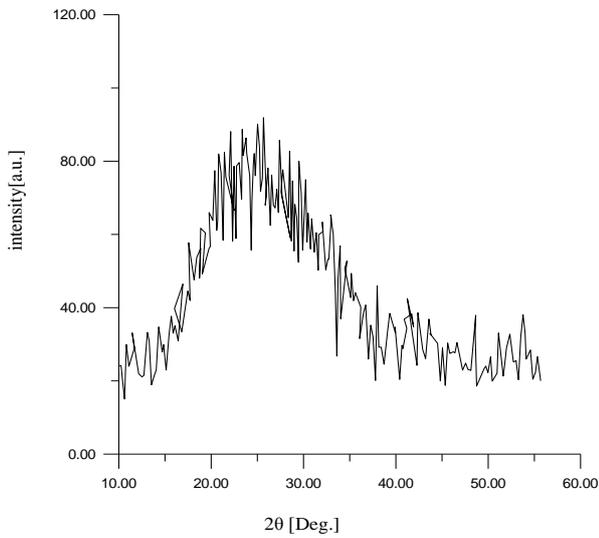
Figure (6) XRD spectra of TiO<sub>2</sub> deposited at sputtering pressure(2.8 pa) and O<sub>2</sub>/Ar percentage (25%).
