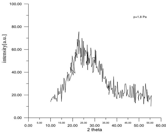
Fig. (2) XRD spectra of TiO<sub>2</sub> deposited at sputtering pressure(1.8 pa) andO<sub>2</sub>/Ar percentage (5%).
