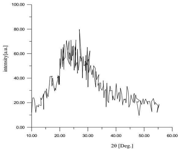
Fig. (3) XRD spectra of TiO<sub>2</sub> deposited at sputtering pressure(2.8 pa) andO<sub>2</sub>/Ar percentage (5%).
