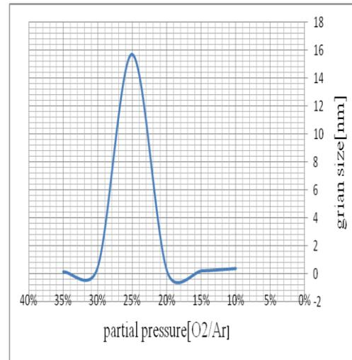
Figure (8) size as a function of partial pressure [ O<sub>2</sub>/Ar ] at sputtering pressure (2.8 pa).
