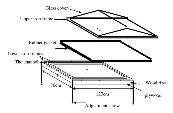
Fig.(1): Schematic diagram of the solar still
