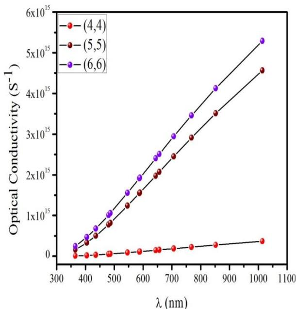
Fig.8 The wavelength versus Optical conductivity
