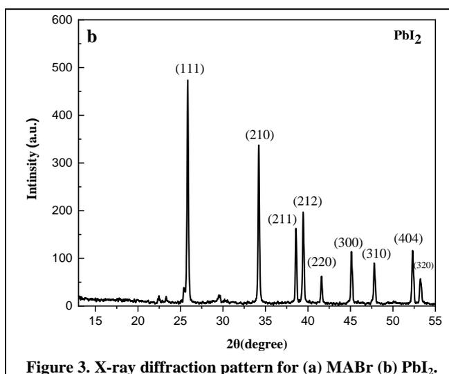
**Figure 3. X-ray diffraction pattern for (a) MABr (b) PbI<sub>2</sub>.**
