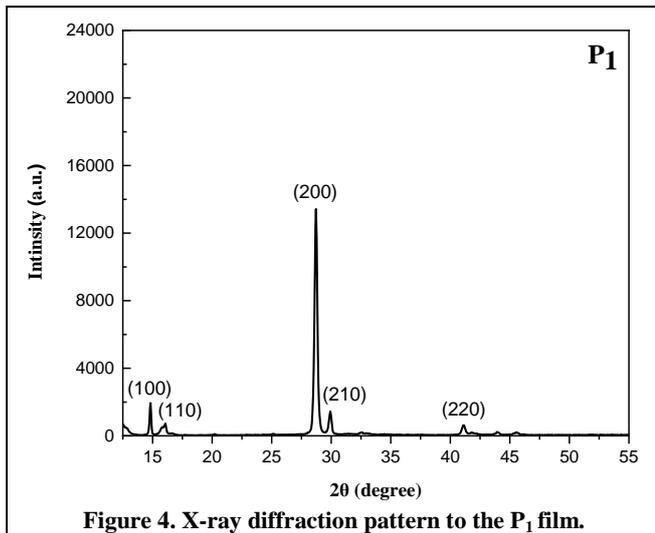
Figure 4. X-ray diffraction pattern to the P<sub>1</sub> film.
