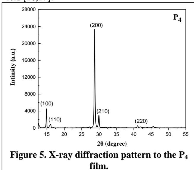
Figure 5. X-ray diffraction pattern to the P<sub>4</sub> film.
