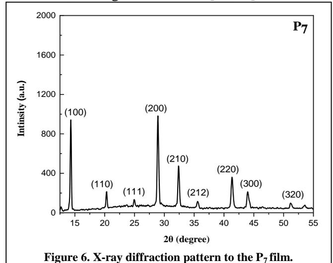
Figure 6. X-ray diffraction pattern to the P<sub>7</sub> film.
