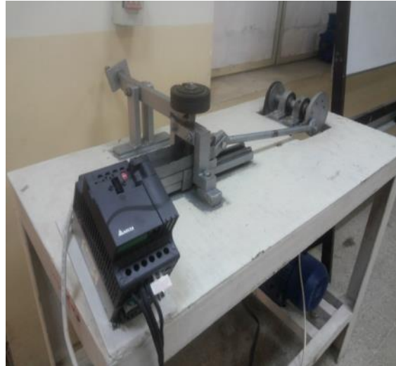
Fig. 7. Reciprocating wear test device.
