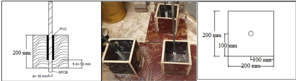
Fig. 5. Bonding test models and Their Details.
