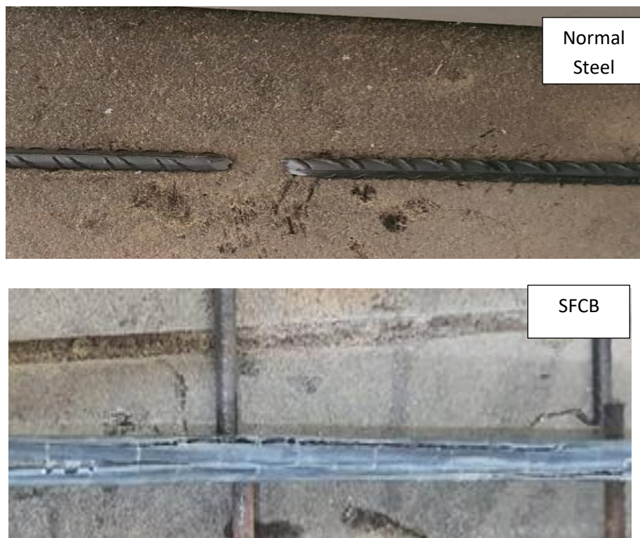
Fig. 7. Failure modes of Normal Steel bar and SFCB Respectively.
