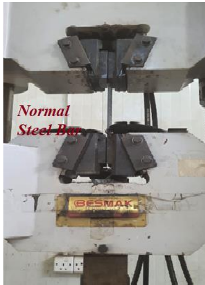
Fig. 3. Testing Machine and Tested Normal Steel Bar.
