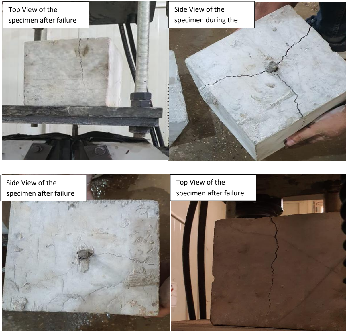
Fig. 10. Failure Mode of The Normal Concrete Specimens of Bonding Test.
