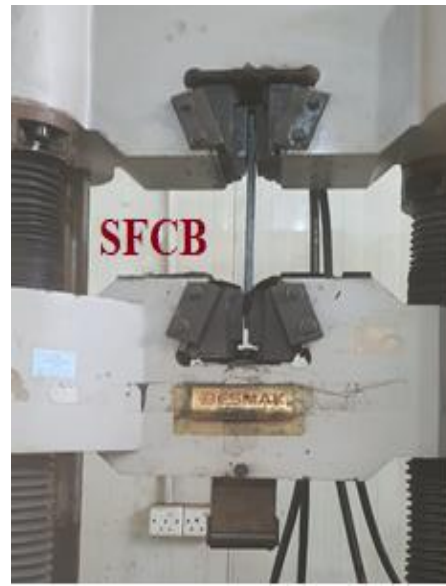
Fig. 4. Testing Machine and Tested SFCB.
