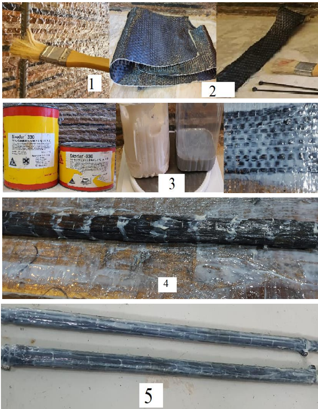
Fig. 2. The Steps of SFCB production process.
