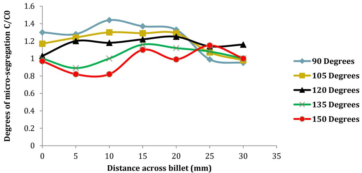
Fig. 3. Effect of variation of runner angle on degree of segregation of Al 5 wt. % Zn.
