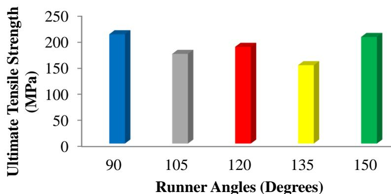
**Fig. 8. Ultimate tensile strength for Al 6wt. % Cu, Al 5wt. % Zn alloy for varied runner angles.**
