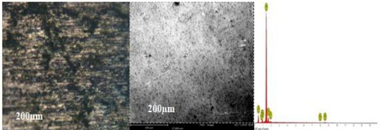
**Fig. 5. Optical micrograph, SEM and EDS of Al 5 wt.% Zn at 1200.**
