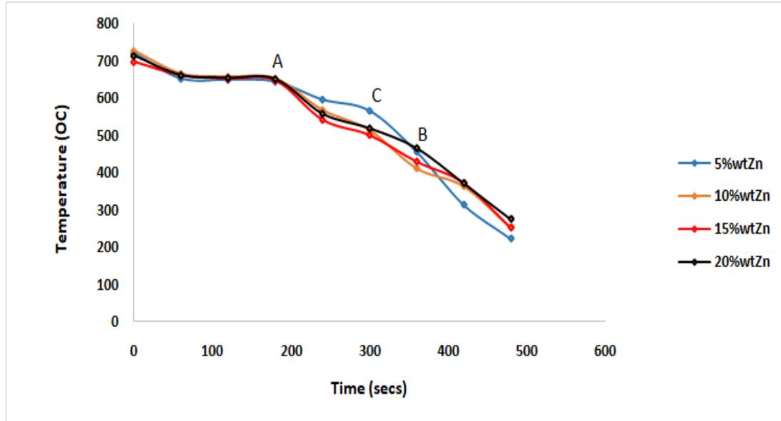
**Fig. 2. Cooling curves for Al-Cu alloy.**
