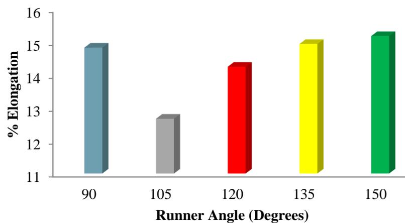
**Fig. 9. Percent elongation for Al 6wt. % Cu, Al 5wt. % Zn alloy for varied runner angles.**
