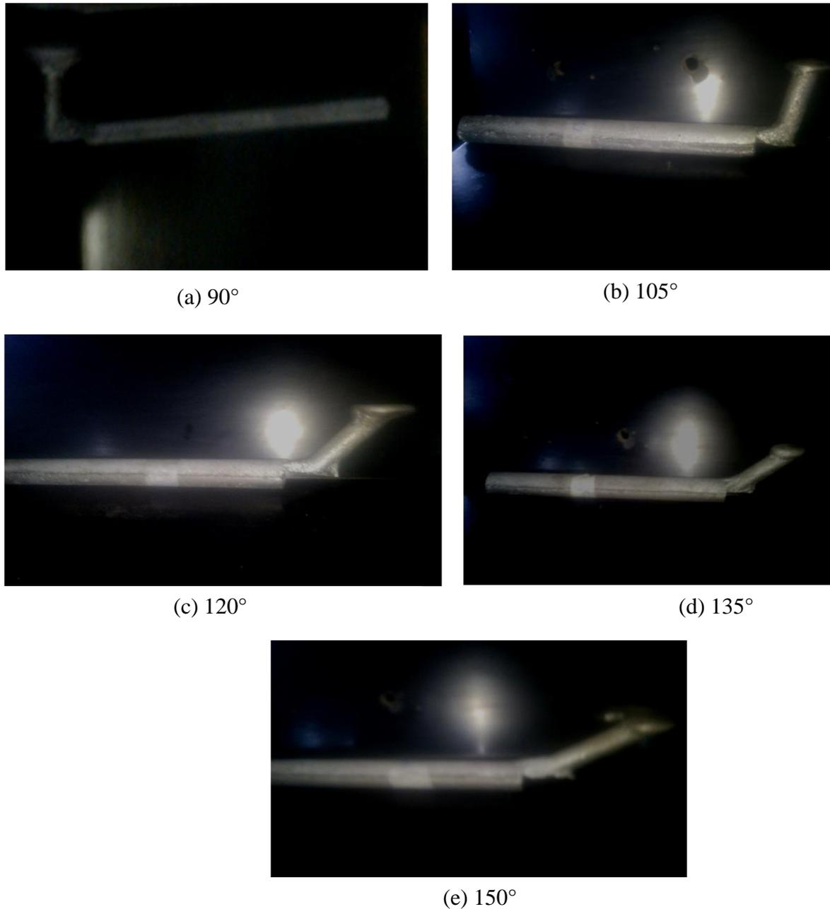
**Fig. 1. Cast samples at varied runner angles.**
