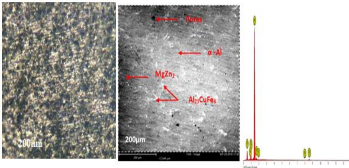
Fig. 4. Optical micrograph, SEM and EDS of Al 5 wt.% Zn at 90°
