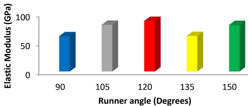
**Fig. 7. Modulus of Elasticity for Al 6wt. % Cu, Al 5wt. % Zn Alloy for Varied Runner Angles.**
