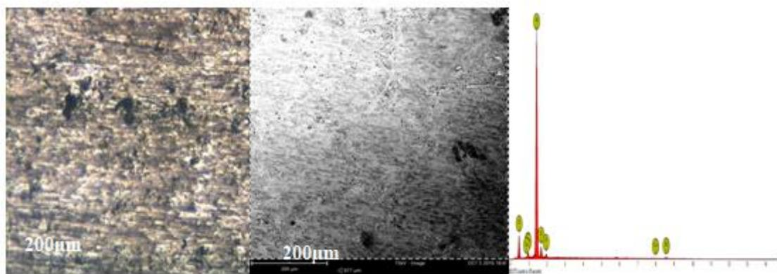
**Fig. 6. Optical micrograph, SEM and EDS of Al 5 wt. % Zn at 150°**
