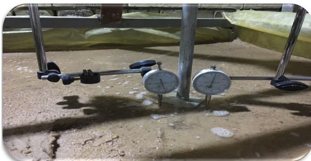
Fig. 7. Failure shape of the natural soil loaded in soaked state.
