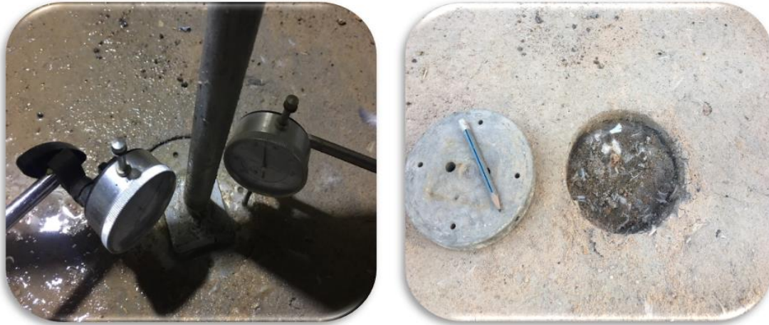
Fig. 8. Failure shape of the treated soil loaded in soaked state.
