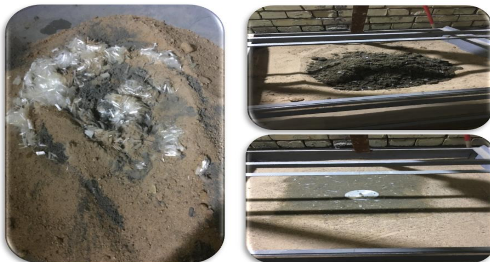
Fig. 5. Preparing treated soil with PPF and cement.
