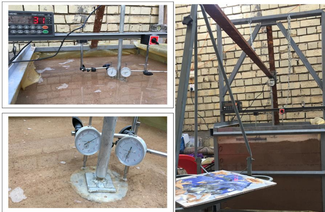
Fig. 4. Saturated soil Prepared for model test with applied the first load increment.
