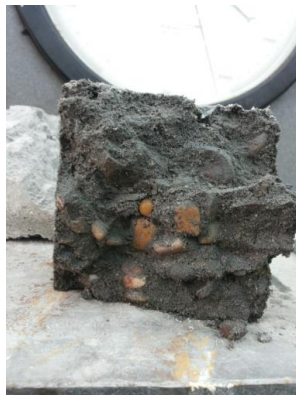
Picture 2. Samples containing (water absorption polymers) cured in Air: a-after 28 days b- after 60 days c- after 90 days d- after 120 days
