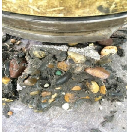
Picture 4. Polymer balls shrinks and exploded leaving pores in concrete.
