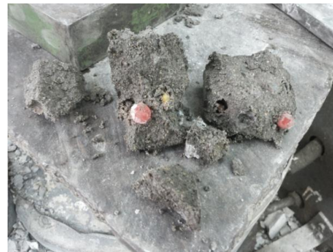
Picture 2. Samples containing (water absorption polymers) cured in Air: a-after 28 days b- after 60 days c- after 90 days d- after 120 days
