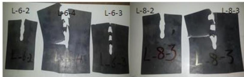
**Fig. 8. Tear-out failure of specimens of L series.**
