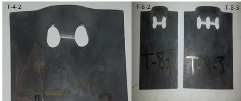
**Fig. 5. Block shear failure of specimens of T serie.**
