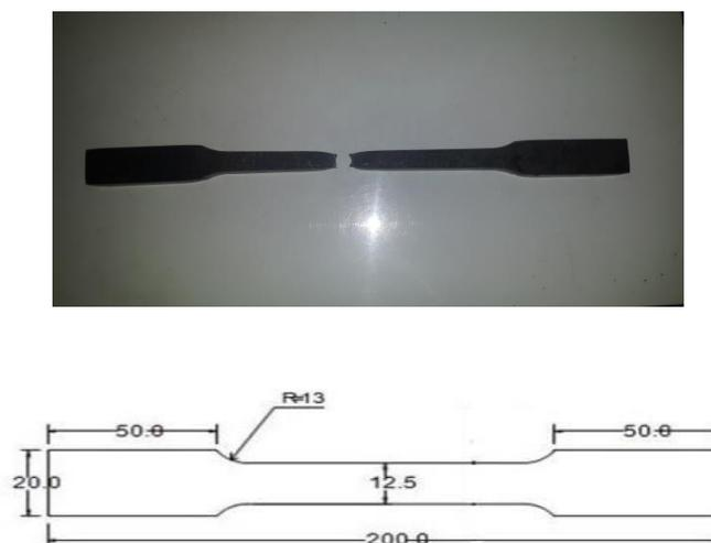
**Fig. 1. Shape and Dimensions of Test Sample.**
