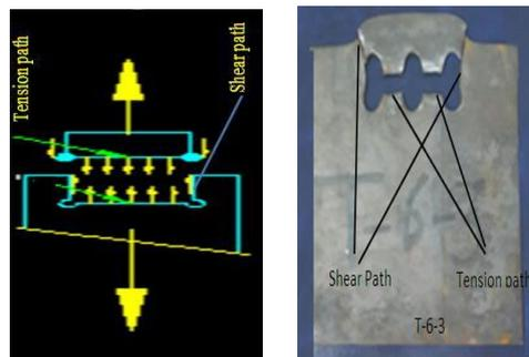
**Fig. 6. Blok Shear Rupture in a Digram and plate T-6-3.**
