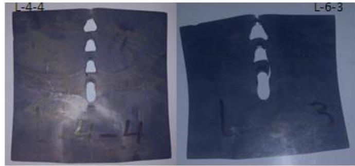
**Fig. 7. Tear-out failure of specimens of L series.**
