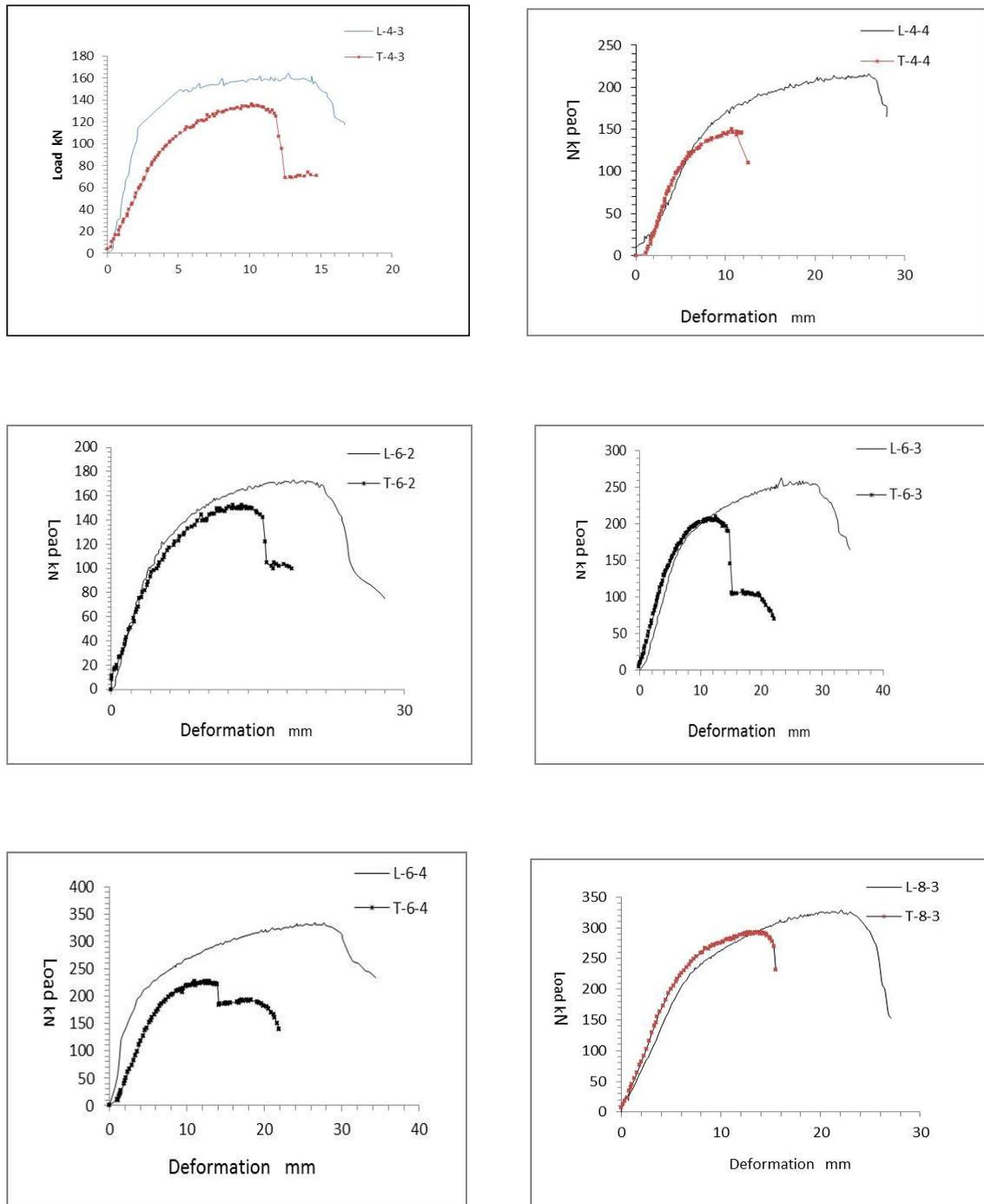
**Fig. 4. Load-Deformation Curves of Specimens of Series Land T.**
