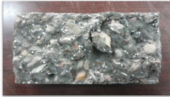
Fig. 5. Split tensile test specimens after test.
