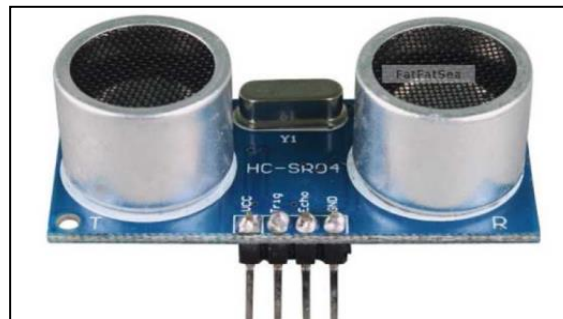
Fig. 6. Ultrasonic Ranging Module HC-SR04 Sensor.
