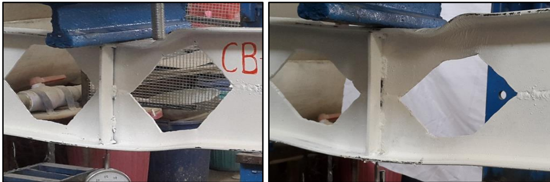
Fig. 4. Typical failure mode of CSBs.
