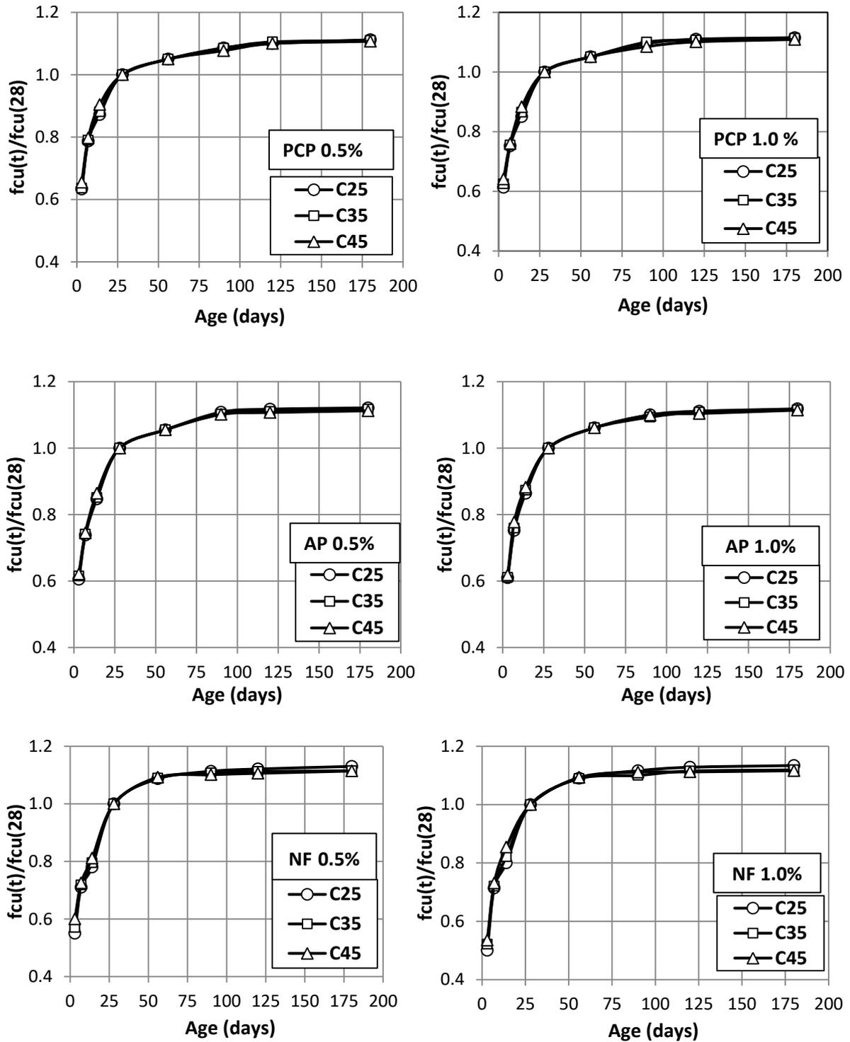
Fig. 3. Effect of SP type with different dosages on  $f_{cu}(t)/f_{cu}(28)$  ratio at different compressive strengths.
