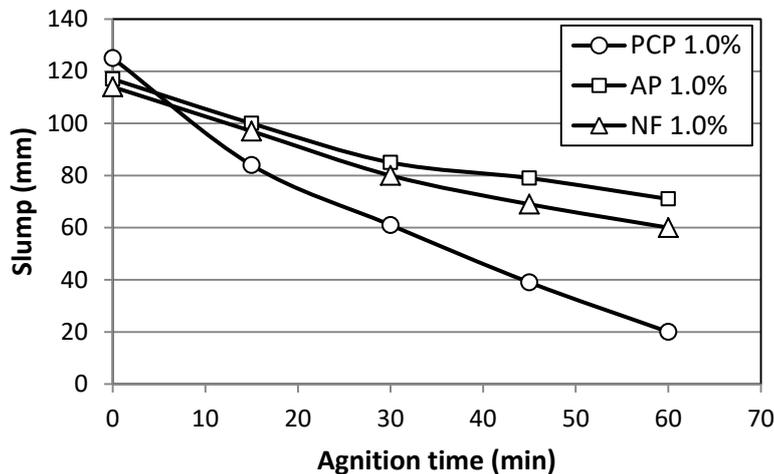
Fig. 1. Slump-loss of superplasticized concrete with W/C ratio of 0.46 and superplasticizer dosage of 1.0% of cement weight.
