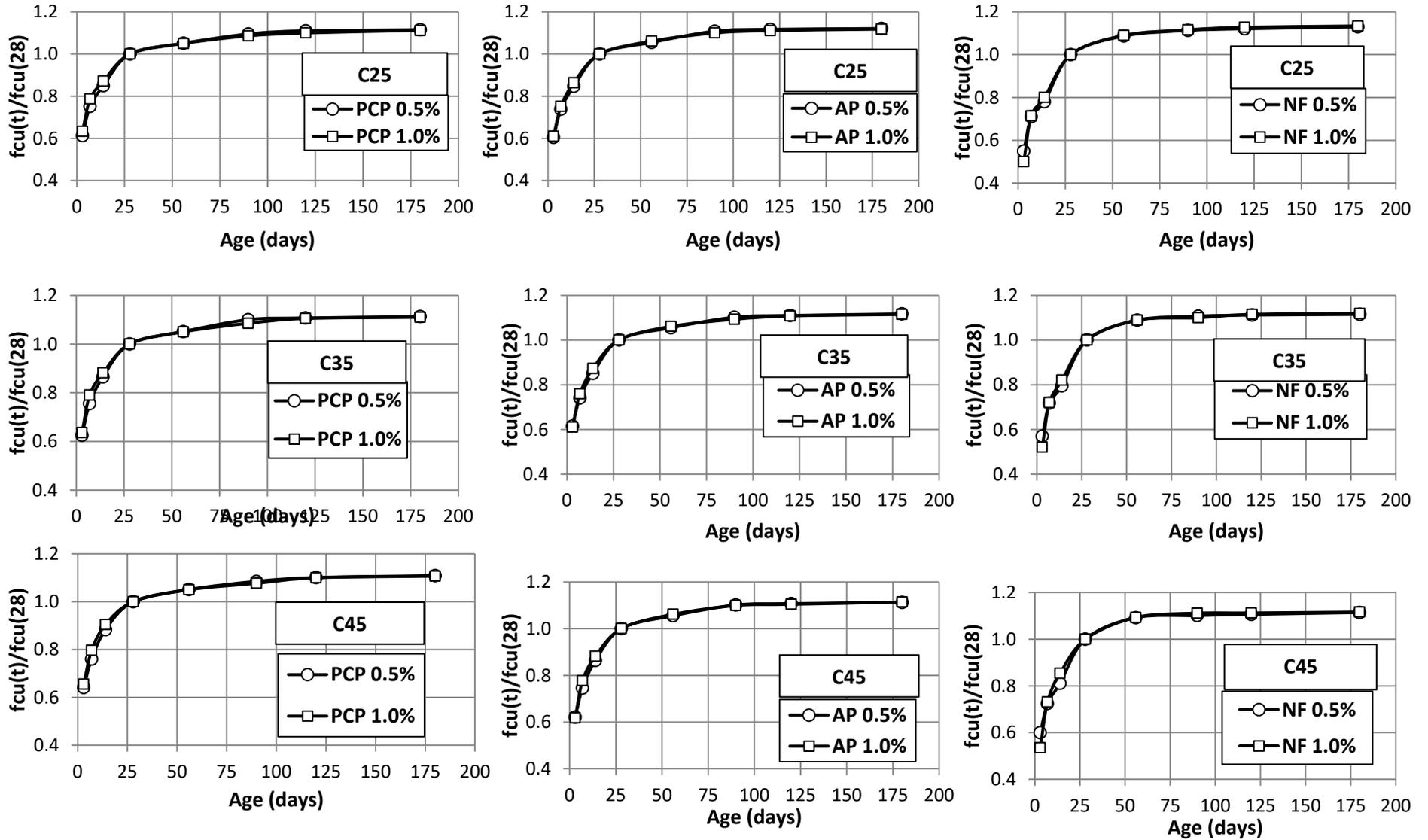
Fig. 4. Effect of dosage of different types of SP on  $f_{cu}(t)/f_{cu}(28)$  ratio at different compressive strengths.
