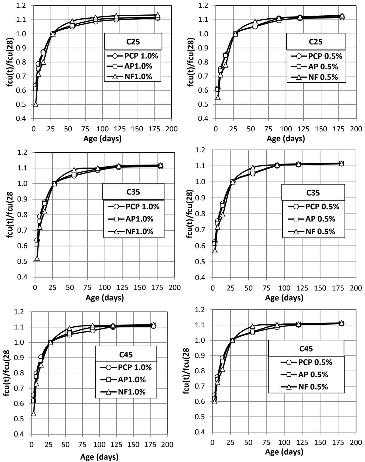
Fig. 2. Effect of SP type with different dosages on  $f_{cu}(t)/f_{cu}(28)$  ratio at different compressive strengths.
