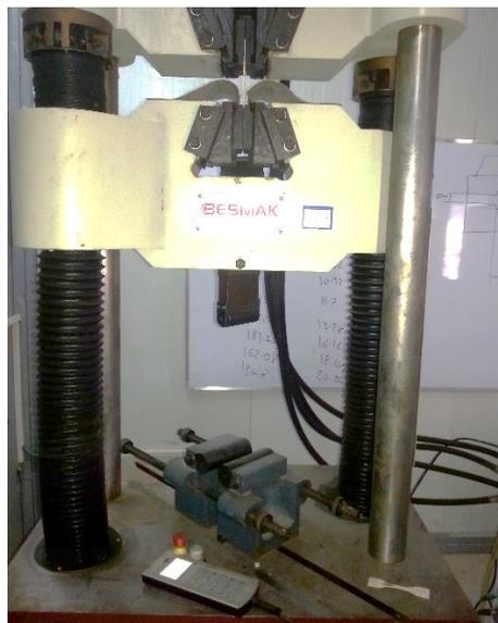
**Fig. 2. Tensile test computerized machine**
