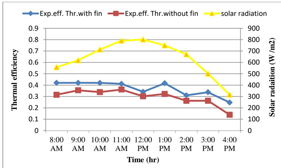
Fig. 5. the variation of thermal efficiency with time day for May 2023, for PV /T module without fins and with fins.
