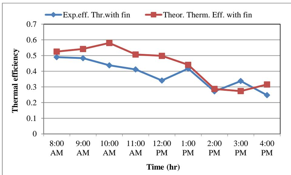
**Fig. 12. Theoretical and Experimental Results of Thermal efficiency for May 2023, for PV /T module with fin.**
