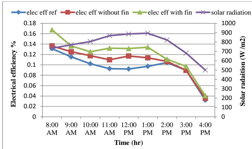
**Fig. 6. The experimental Electrical efficiency and solar radiation for May 2023, for PV module and PV/T module without fins and with fins.**
