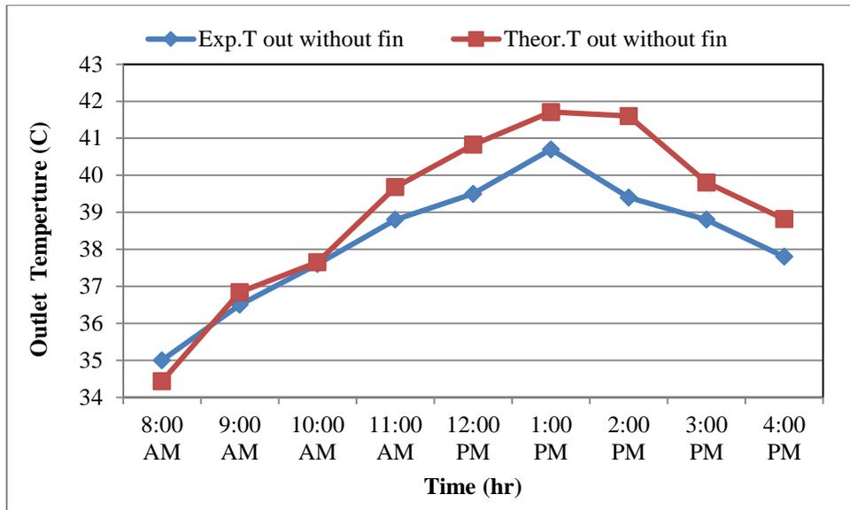
**Fig. 11 Theoretical and Experimental Results of Outlet Temperature for May 2023, for PV /T module without fin.**
