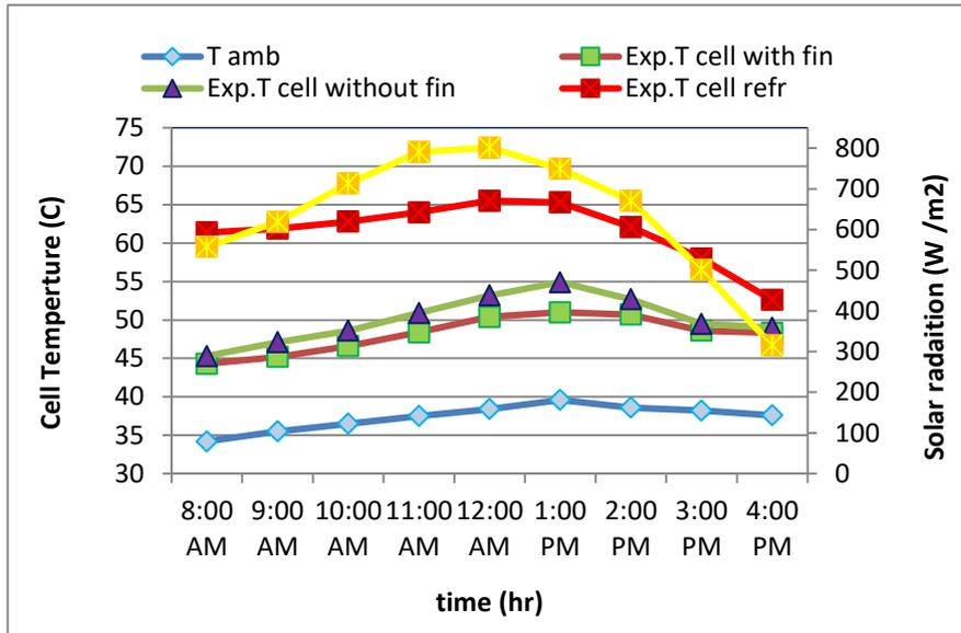
Fig. 4. The experimental variation of PV temperature with time day for 15 May 2023, for PV module, PV/T module and PV /T module with fin
