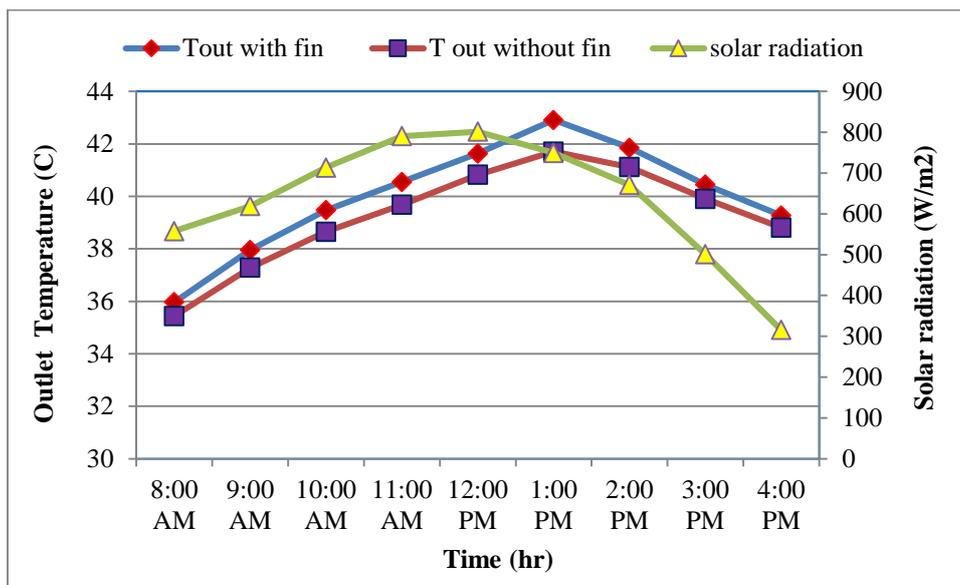
**Fig. 8. the variation of outlet temperature with time day for May 2023, for PV /T module and PV /T module with fin.**
