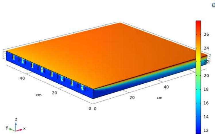
**Fig.1. Domain temperature with fin**
