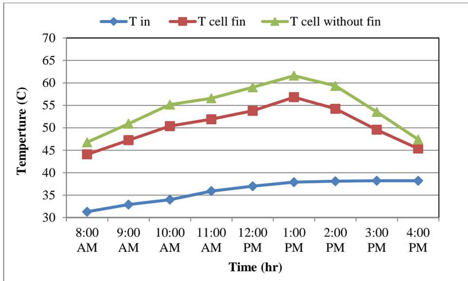
**Fig. 7. the theoretical variation of Cell temperature with time day for May 2023, for PV /T module and PV /T module with fin.**
