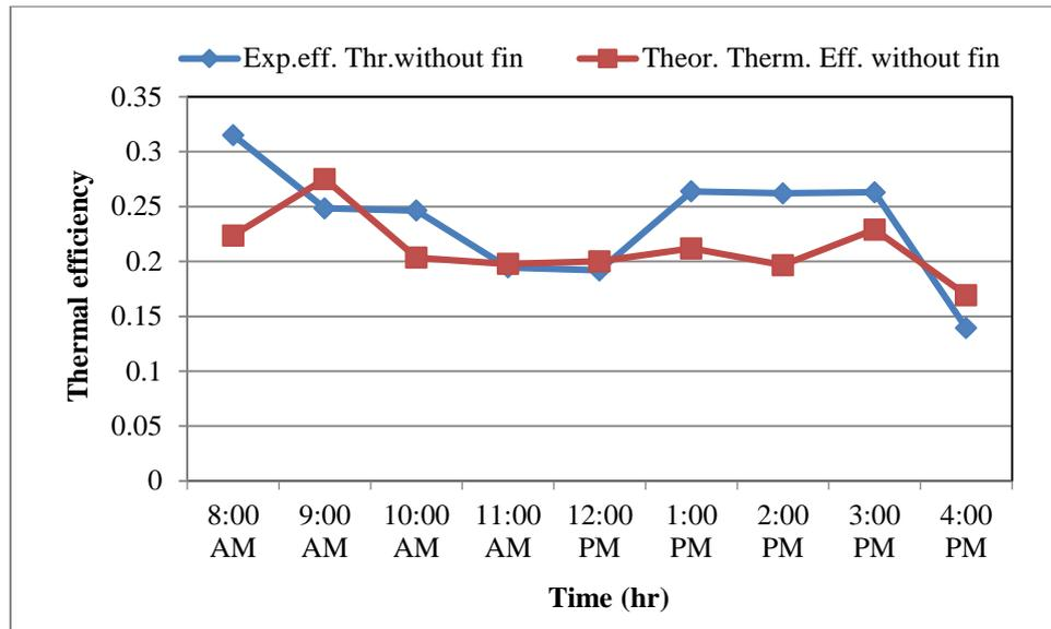
**Fig. 13. Theoretical and Experimental Results of Thermal efficiency for May 2023, for PV /T module without fin.**
