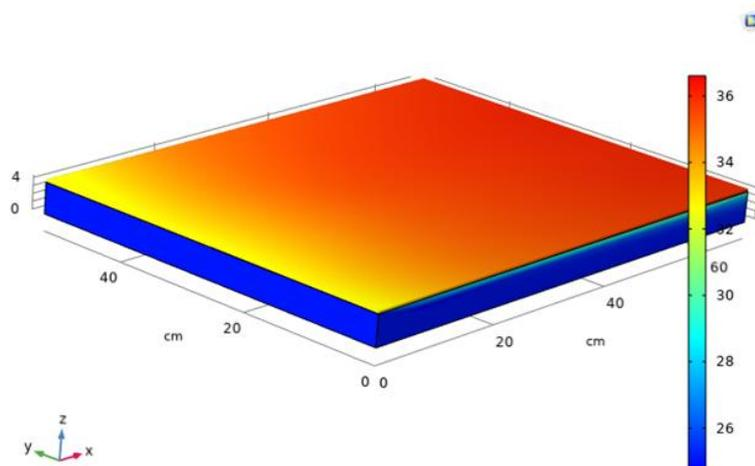
**Fig.2. Domain temperature without fin**
