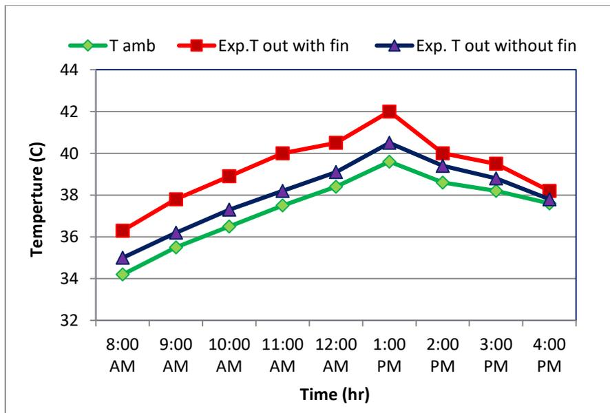
Fig. 5. the variation of outlet temperature with time day for May 2023, for PV /T module and PV /T module with fin.
