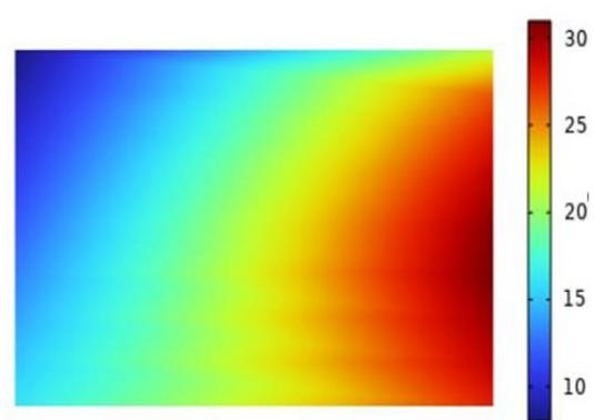
**Fig. 9b back sheet surface temperature with fins.**
