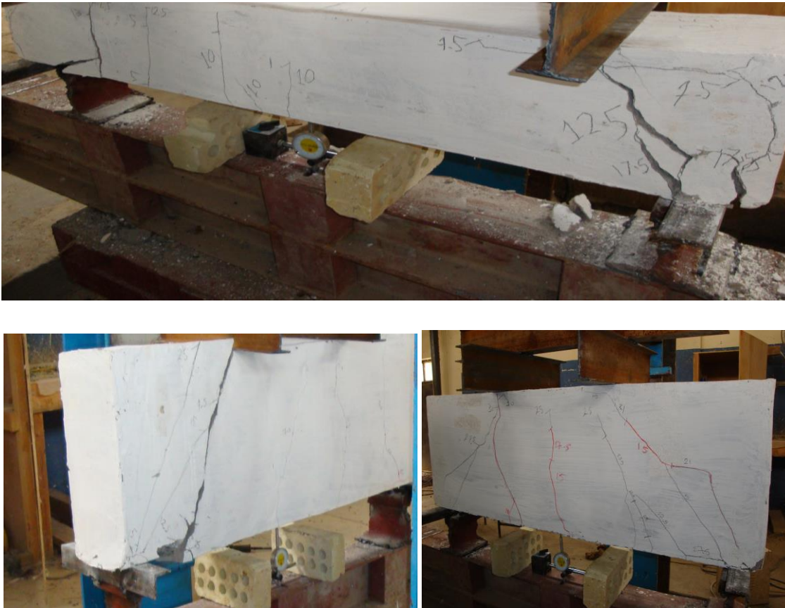
Fig.(6)Shear crack pattern for Monopanel beam specimens
