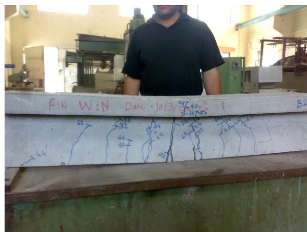
Fig.3 Cracks pattern of beam B2
