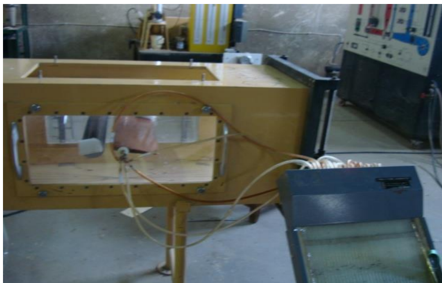
Fig.8 Manometer used to Measure the Static Pressure around Airfoil
