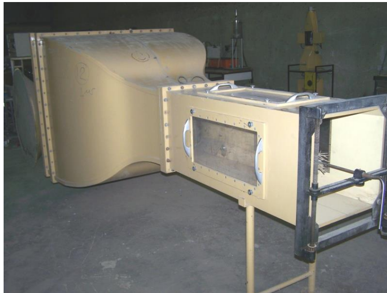
Fig.3 Subsonic Wind Tunnel.
