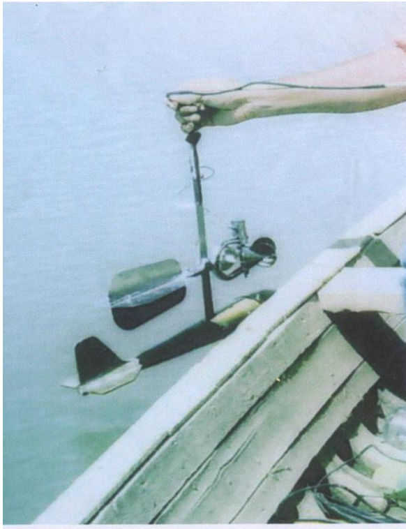
Plate 2. Velocity computations using current meter in Al-Kufa river
