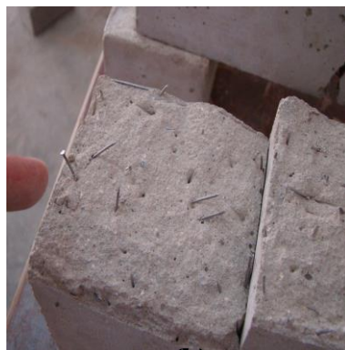
Photo 1, (a) Fibrous mortar beams at failure (no complete separation) , (b) Randomly distributed fibers throughout the beam section, and (c) Plain mortar beam at failure (completely separation)
