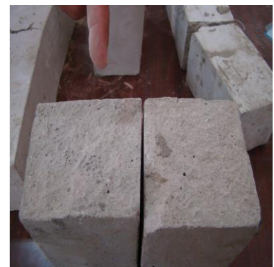
Photo 1, (a) Fibrous mortar beams at failure (no complete separation) , (b) Randomly distributed fibers throughout the beam section, and (c) Plain mortar beam at failure (completely separation)
