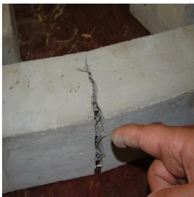
Photo 1, (a) Fibrous mortar beams at failure (no complete separation) , (b) Randomly distributed fibers throughout the beam section, and (c) Plain mortar beam at failure (completely separation)
