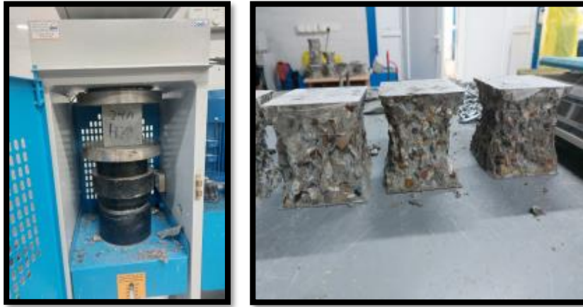
Fig. 7. Compressive strength test and failure mode of specimens
