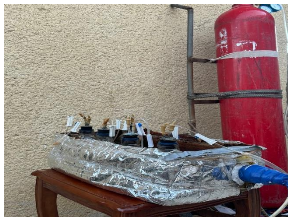
Fig. 2. Experimental setup for Biogas production system
