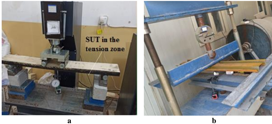
Fig. 3. a. Four-points loading test setup, b. Three-points loading test setup.
