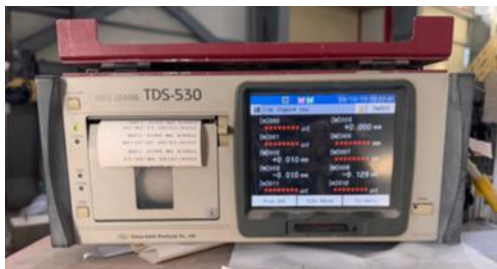
Fig. 4. Data logger used for control the loading and measuring the deflection in slab.
