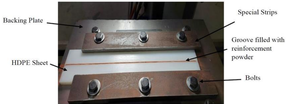
Fig. 2. HDPE sheet clamping system
