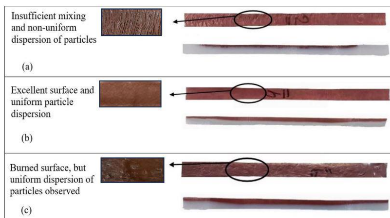
Fig. 6. Surface and cross section of composites at (a) low rotational speed (b) medium rotational speed (c) High rotational speed.
