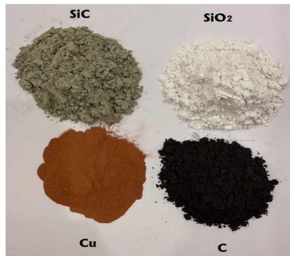
Fig. 1. Reinforcement powders materials
