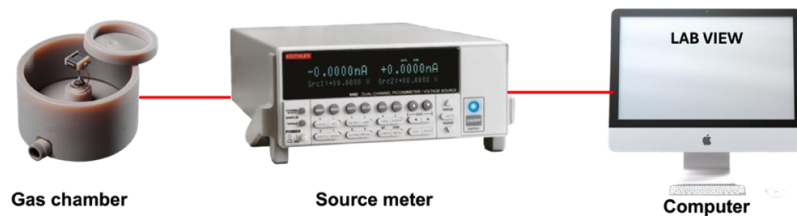
Fig. 3 The I-V measurement setup, which includes a gas chamber containing the interdigitated electrode (IDE), source meter, and a LabView platform on the computer.
