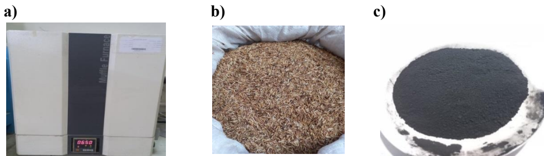
Fig. 1. RHA Productions: (a) The furnace used, (b) Raw rice husks, (c) RHA after grinding
