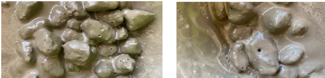
Fig. 6. The holes appeared during the coating process with the ratios (750) and (1000)
