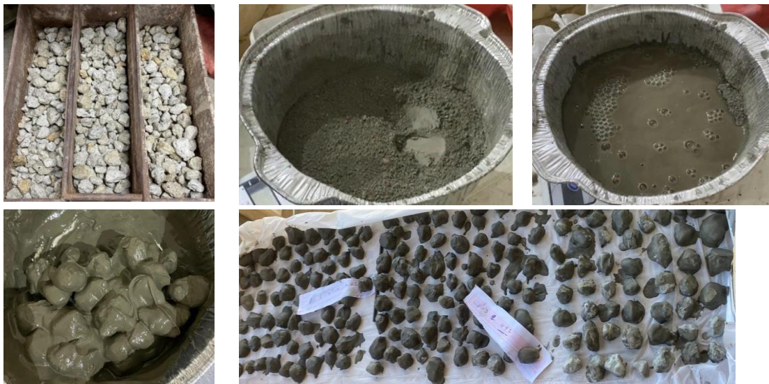
Fig. 2. Pumice preparation, coating mixture, and pumice particles after coating
