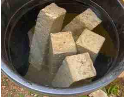
Fig. 2a. Samples exposed to Corrosive environment
