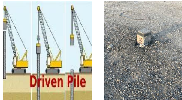
Fig. 1. driven pile installation
