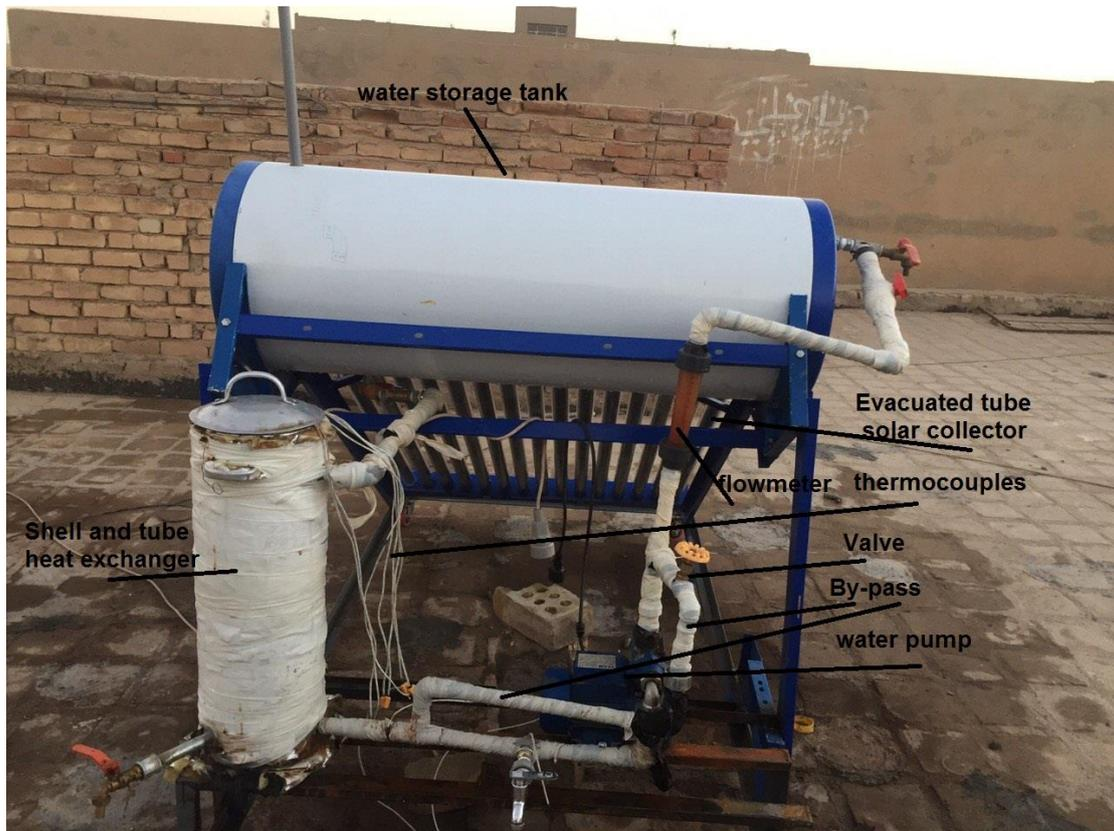
**Fig. 1. The experimental rig.**
