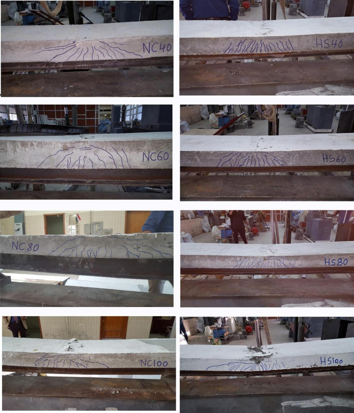
Fig. 5. Mode of failure and crack pattern for tested specimens.
