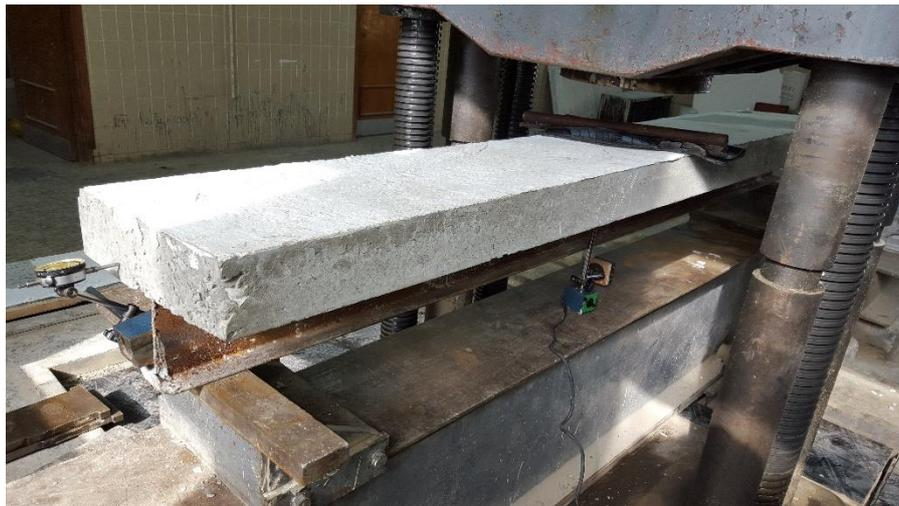
**Fig. 4. Steel concrete composite beam specimen under test.**
