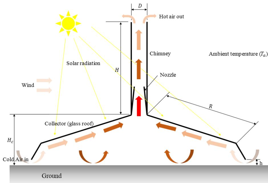
Fig. 1. Schematic diagram of solar chimney.
