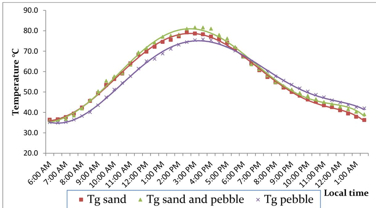
**Fig. 8.** The influence of various ground types on the surface ground temperature.
