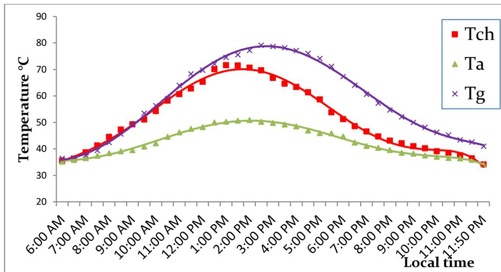
Fig. 5. Ground, chimney and ambient temperatures verse time for sand basement.
