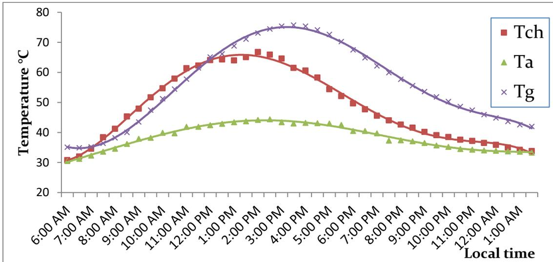
**Fig. 7. Ground, chimney and ambient temperatures verse time for black pebble basement.**
