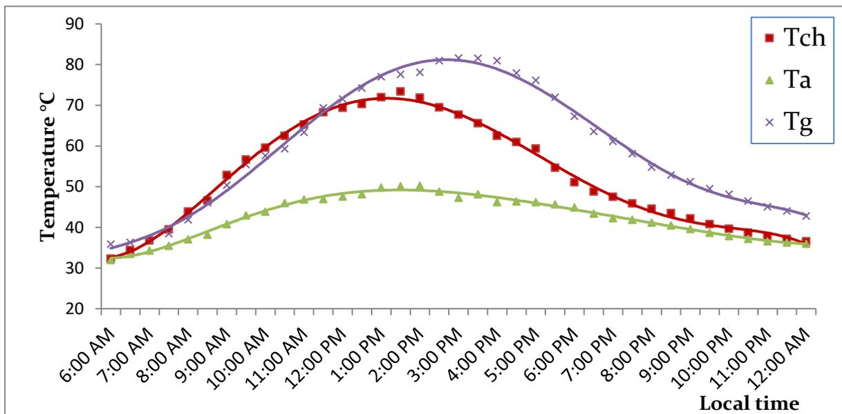
**Fig. 6. Ground, chimney and ambient temperatures verse time for mixed basement (sand and black pebble).**
