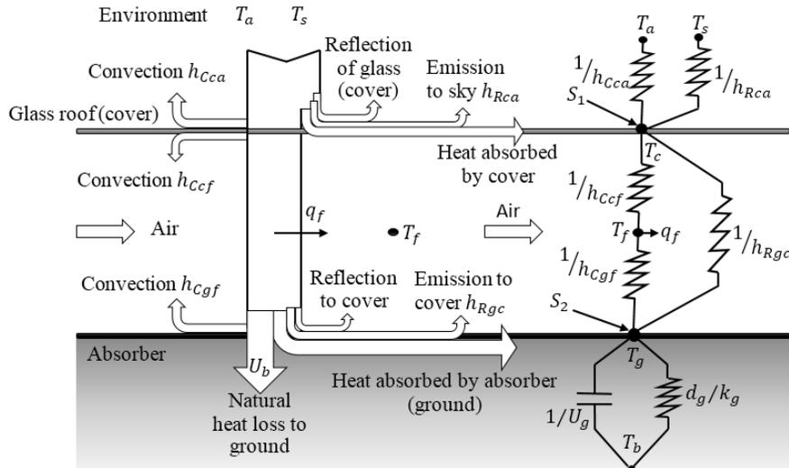
**Fig. 4. Thermal network for the collector of solar tower.**
