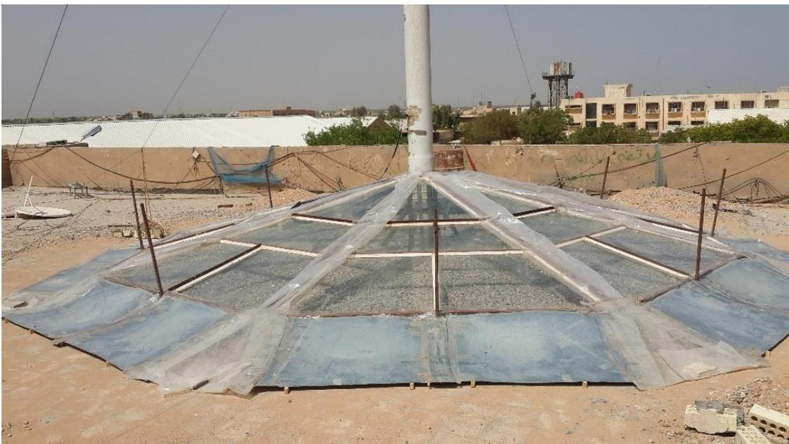
**Fig. 2. Experimental rig of solar chimney.**
