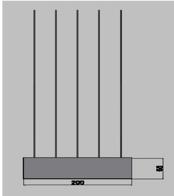
Fig. 7. Pull-out test specimen.
