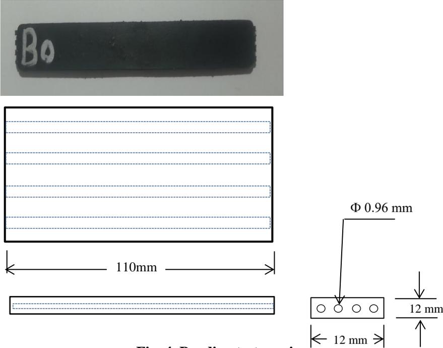
Fig. 4. Bending test specimen.
