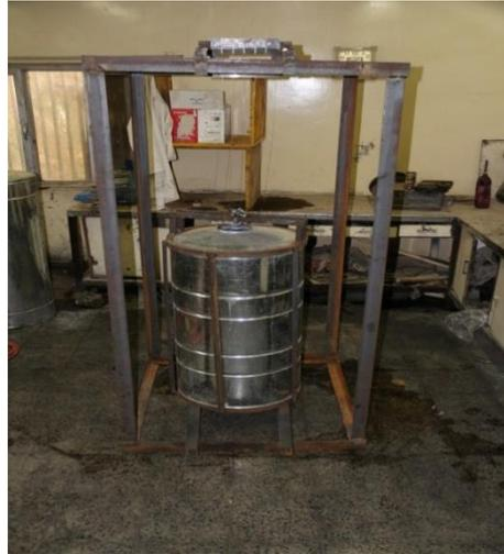
**Fig. 3. The rig for applying pre-tension load on bead wires.**
