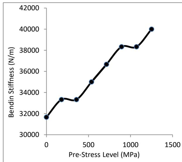
**Fig. 11. The relation between the pre-stress levels and bending stiffness.**
