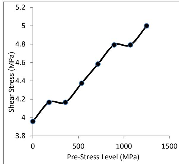
**Fig. 9. The relation between the pre-stress level and the maximum shear stress**
