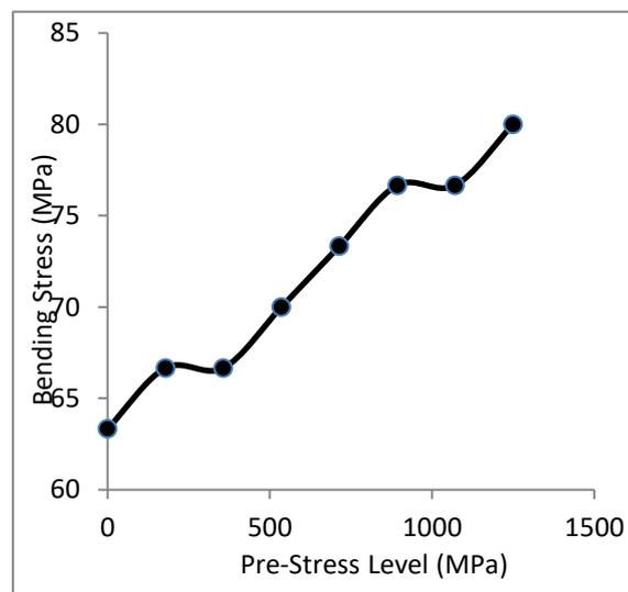
Fig. 8. The relation between the pre-stress level and the maximum bending stress.
