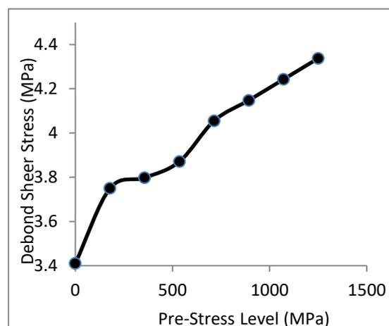
**Fig. 12. The relation between the pre-stress level and the debond shear stress.**
