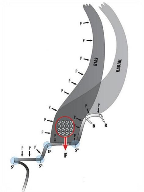
Fig. 2. Bead ply in radial and bias Mounted Tires (WTC, 2017).
