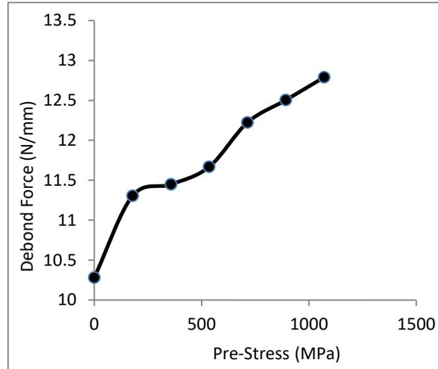
**Fig. 13. The relation between the pre-stress level and the debonding force.**
