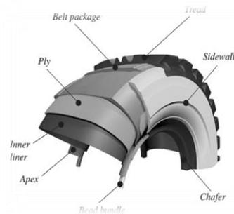
**Fig. 1. The basic construction of the typical tire (Adetan et al., 2008).**
