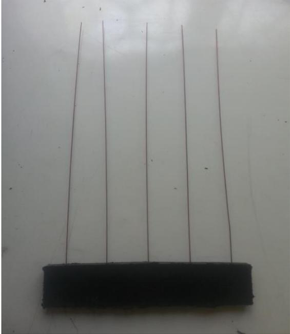
Fig. 6. Pull-out test specimen.
