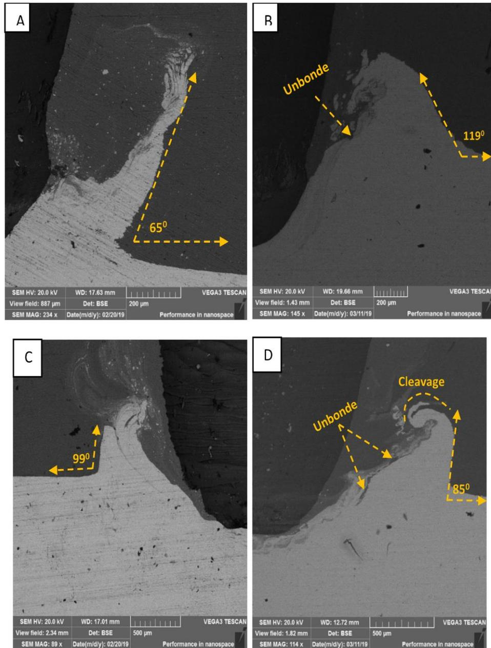
Fig. 6. The SEM photograph of cross section joints were welded by (1400 rpm and 30 sec) (A) without filler (B) with V1-ZnO filler, (C) with V2-ZnO filler and (D) with V3-ZnO filler.
