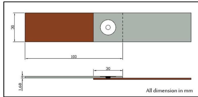
**Fig. 2. The dimensions of dissimilar welding Specimen.**
