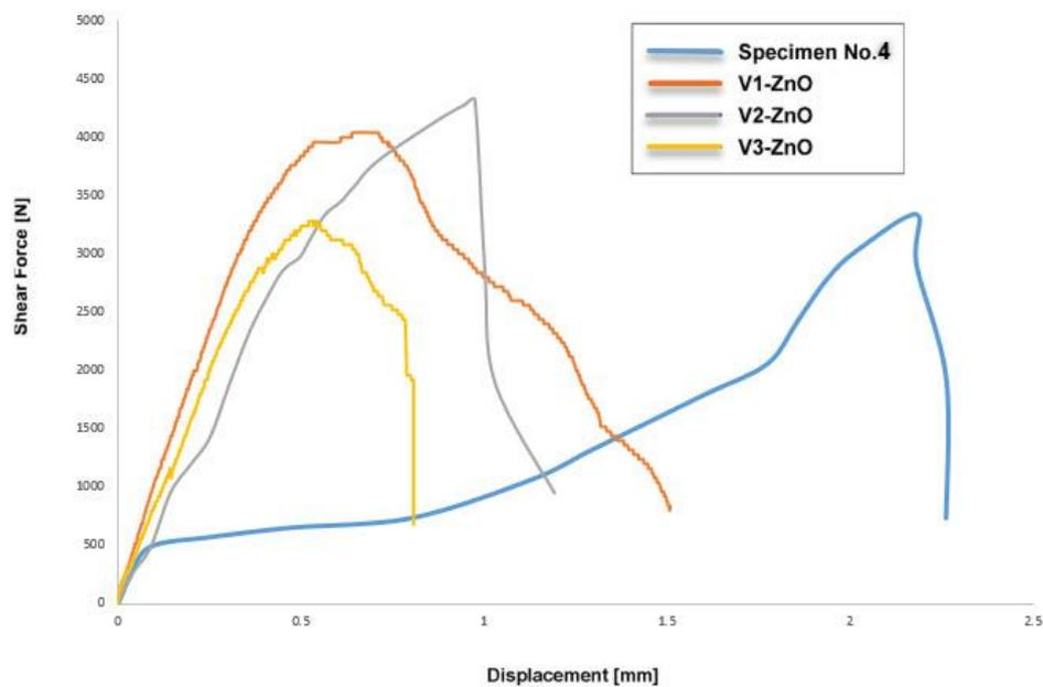
**Fig. 5. The effect of (ZnO) filler content on the behavior of tensile shear load and deflection of joints welded at (1400 rpm) rotation speed and (30 sec) dwell time.**
