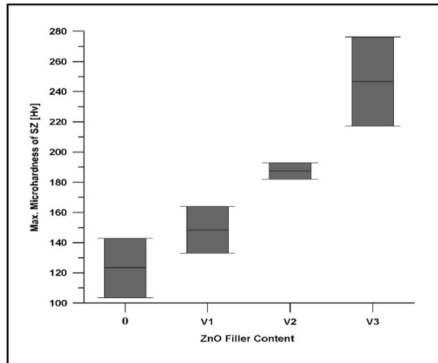
**Fig. 9.** The Microhardness values of SZ with ZnO filler content for FSSW joints that welded at (1400 rpm and 30 sec).
