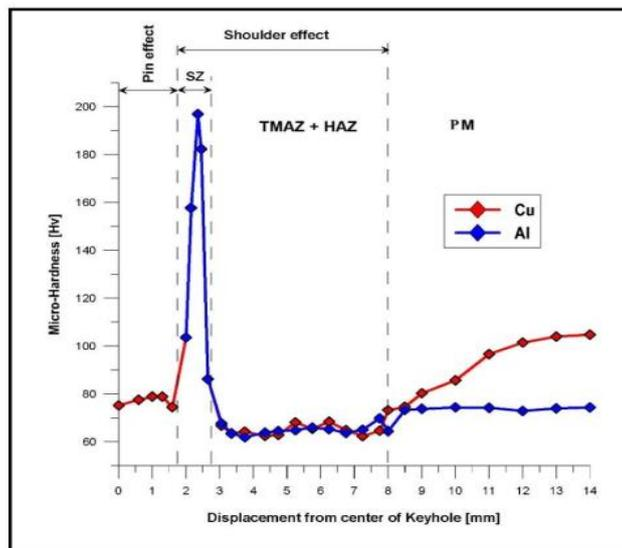
**Fig. 10.** The Vickers microhardness values through the cross section of specimen with V2-ZnO filler that welded at (1400 rpm and 30 sec).
