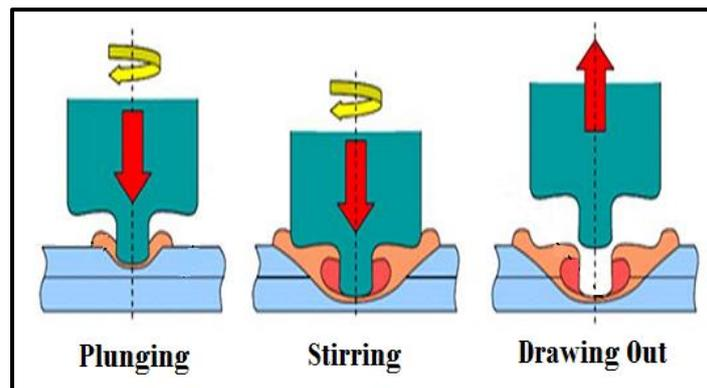
**Fig. 1. Schematic illustration of friction stir spot welding process (Mubiayi & Akinlabi 2015).**
