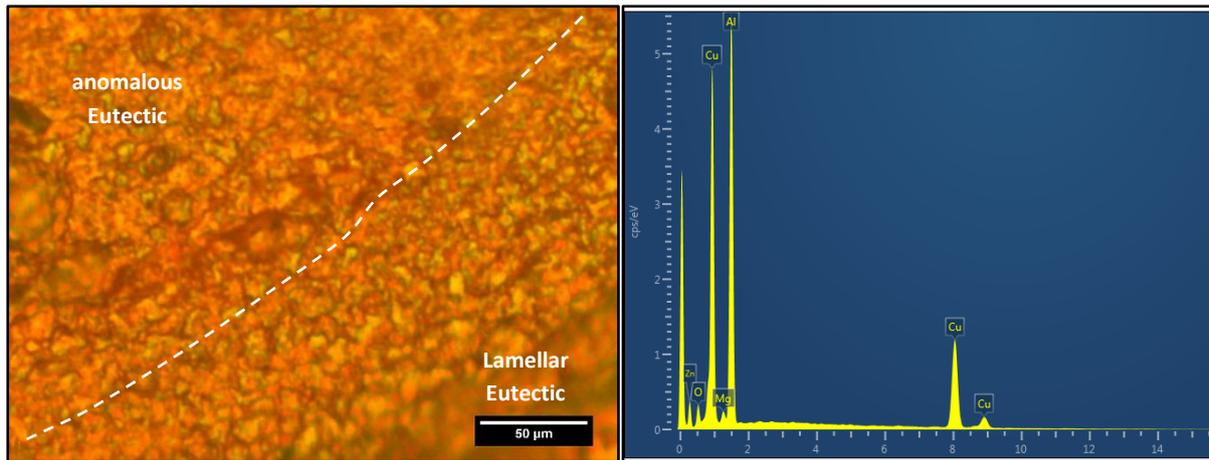
**Fig. 7. The lamellar and anomalous microstructure form of IM layer (left) and the EDS (right) for joint No. C.**
