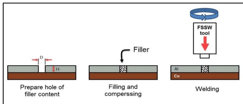
**Fig. 4. Schematic of illustration of adding ZnO filler material between the plates before FSSW.**
