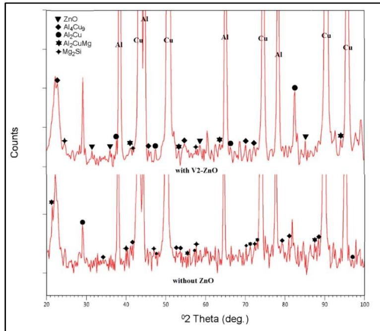
**Fig. 8. The XRD results of the cross section of weld joints that welded at (1400 rpm and 30 sec), with V2 ZnO filler content and without addition filler.**
