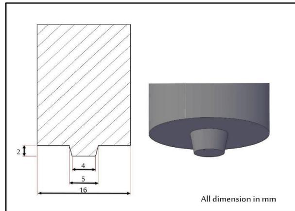
**Fig. 3. The dimensions and geometry of welding tool.**
