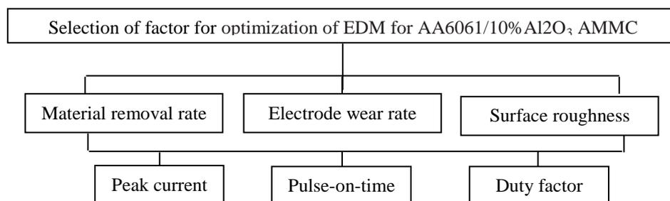
**Fig. 1. Hierarchy of optimization of EDM for AA6061/10%Al<sub>2</sub>O<sub>3</sub> AMMC.**
